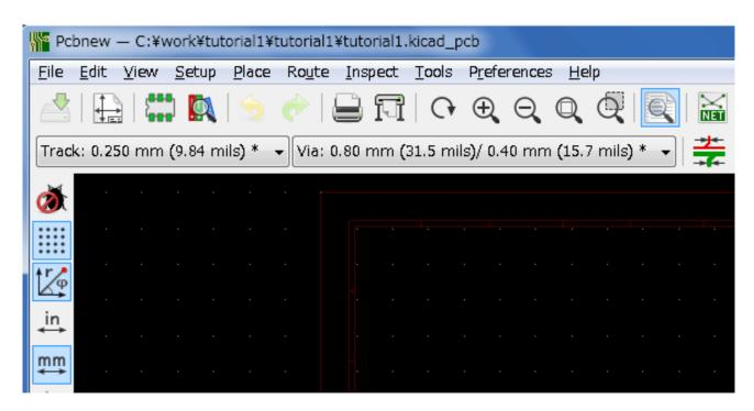
16. If you would like to add more track widths go to: **Setup** → **Design Rules** → **Global Design Rules** tab and at the bottom right of this window add any other width you would like to have available. You can then choose the widths of the track from the drop-down menu while you lay out your board. See the example below (inches).
