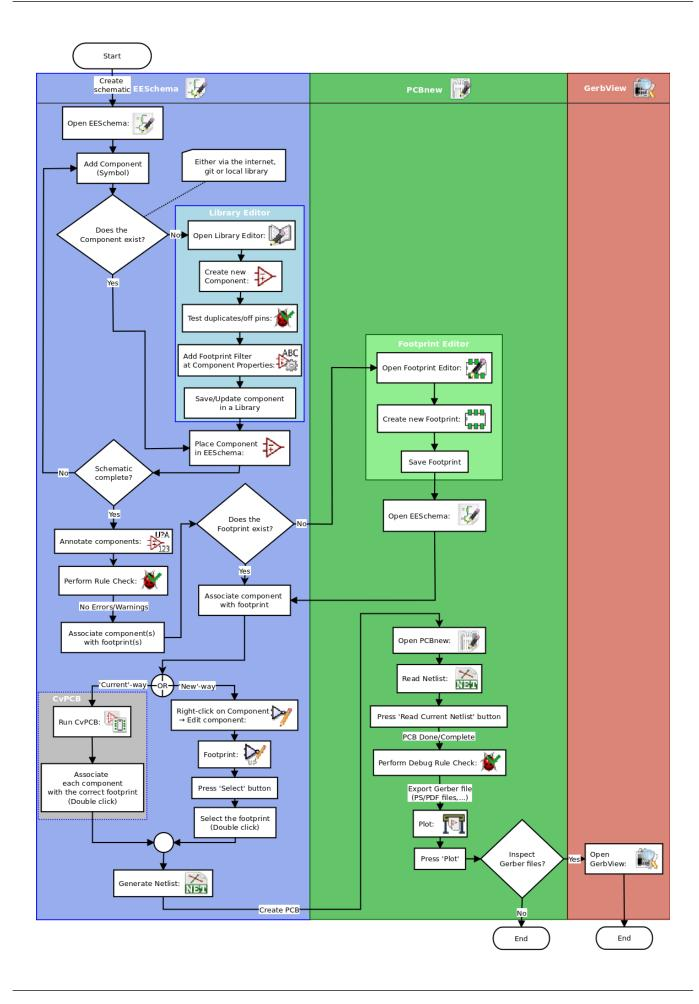
For more information about creating a component, read Making schematic symbols. And for information about how to create a new footprint, see Making component footprints.
