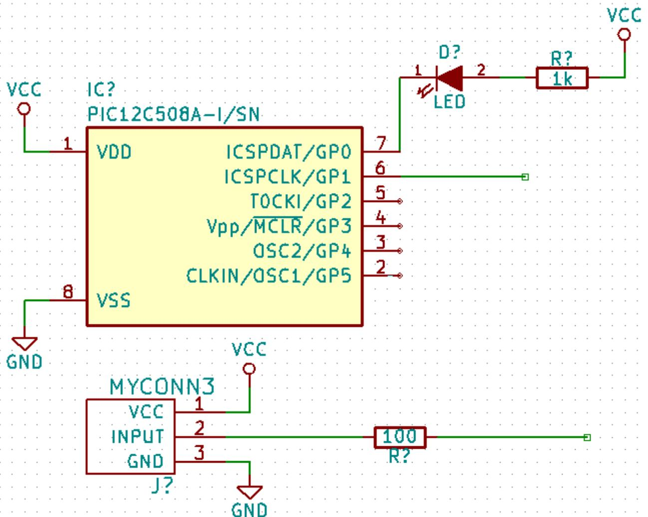
34. We will now consider an alternative way of making a connection using labels. Pick a net labelling tool by clicking on the *Place net name* icon **A** on the right toolbar. You can also use [I].
