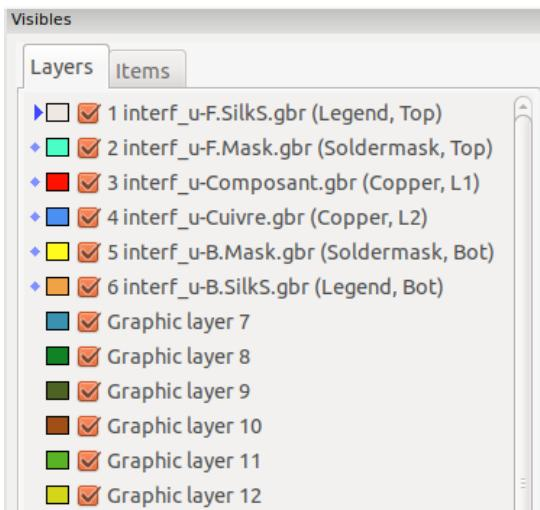
The Layers Manager controls and displays visibility of all layers. An arrow indicates the active layer, and each layer can be shown or hidden with the checkboxes.
