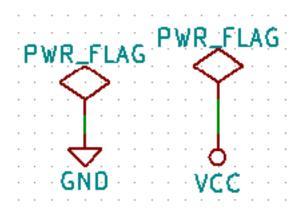
This will avoid the classic schematic checking warning: Warning Pin power\_in not driven (Net xx)
